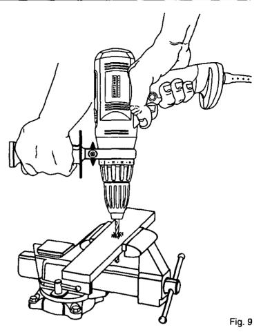
**WARNING:** Be prepared for binding or bit breakthrough. When these situations occur, drill has a tendency to grab and kick opposite to the direction of rotation and could cause loss of control when breaking through material. If not prepared, this loss of control can result in possible serious injury.
